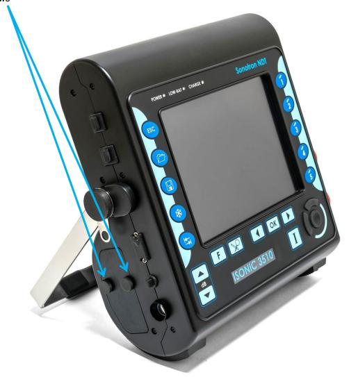
If necessary the internal battery may be charged inside the instrument while it is working. For that purpose the external AC/DC converter / charger should be connected to the appropriate terminal of the instrument and the power cord of the external AC/DC converter should be connected to the mains 100...240 VAC / 40...60 Hz
