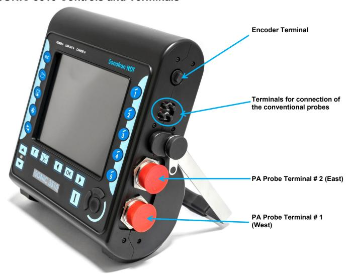
Terminals for connection of the conventional probes
