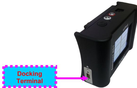
Docking terminal allows keeping the instrument encapsulated into some device, for example PIG (Pipe Inspection Gauge), robotic scanner for tank shell thickness gauging and the like so the full control of the instrument, 9VDC powering, and charging of the internal battery are possible through one connector only
