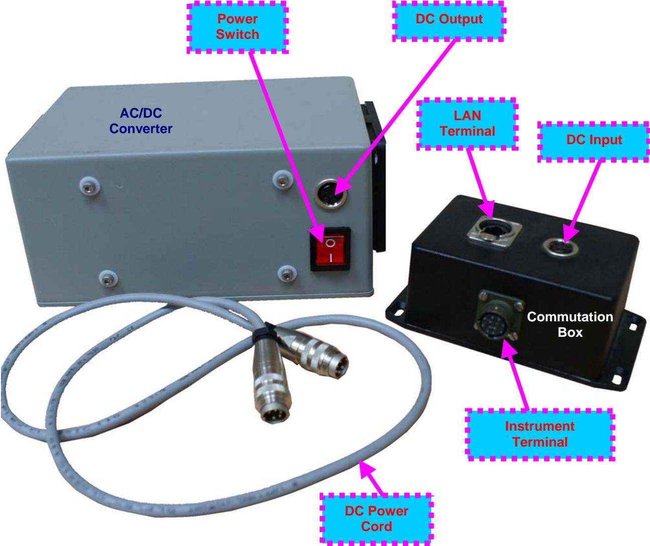
**3.2.4. AC/DC Converter with Built-In Commutation Box – Instruments
