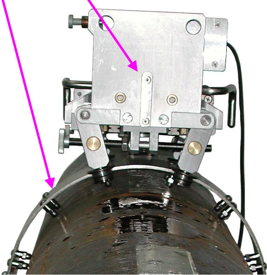
Fit the **frame for carrying probes** into the scanner
