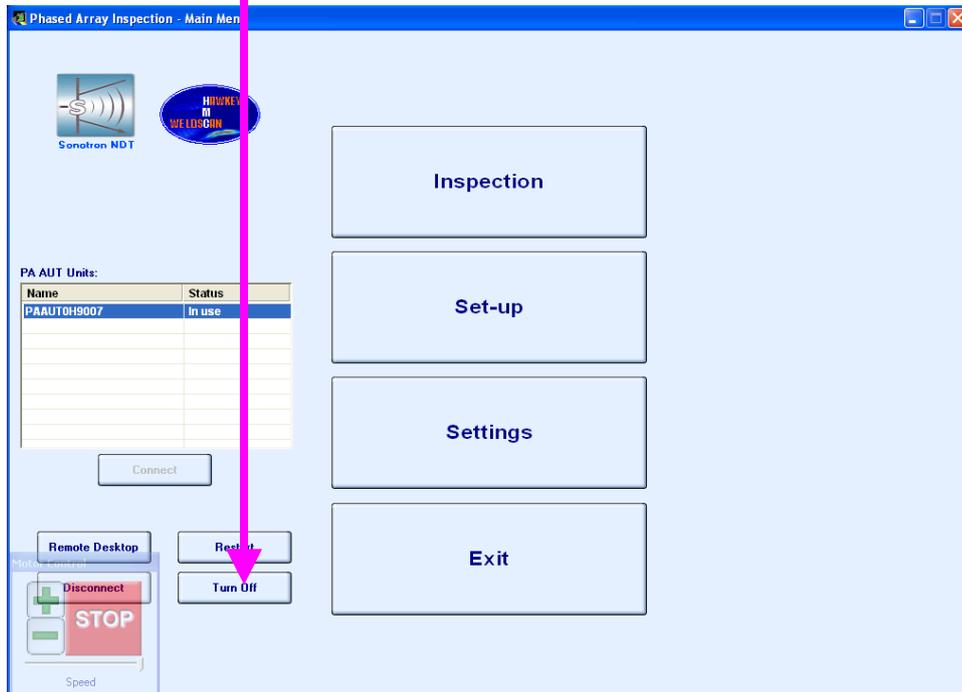
Wait until name of ISONIC PA AUT instrument disappears from the list, then set power switch on the AC/DC converter into **O** position
