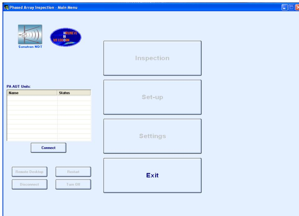
Upon on-board satellite computer of **ISONIC PA AUT** boots up and the hardware initialization is completed the name of the instrument appears in the list and it's status of readiness for the operation is indicated as **Idle**
