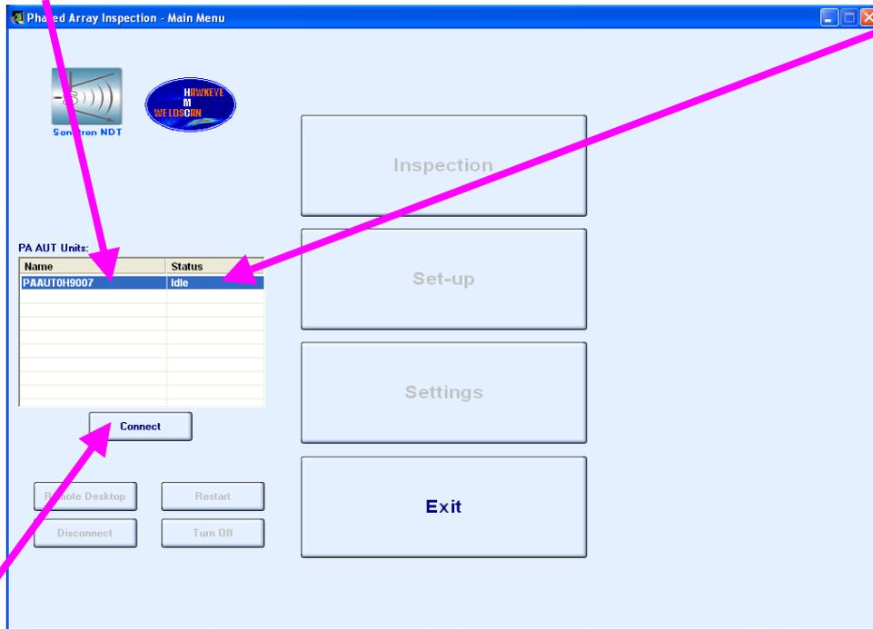
Click on **Connect** to establish communication between remote control computer and **ISONIC PA AUT**, the start-up screen appears then:
