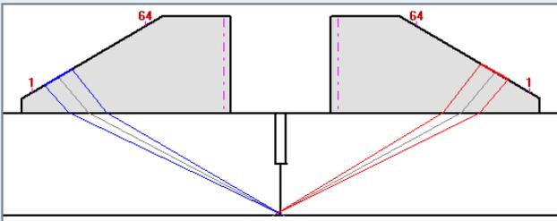
Final screen of *Ultrasonic Setup Wizard* relates to configuration of the *strip chart*. *Strip chart* is a method of AUT data presentation whereas each pulsing-receiving shot is continuously recorded into corresponding strip. Reshaping of *Strip Chart* is possible through manipulating **position / lateral displacement of each strip** according to the probes fitting into the scanning frame:
