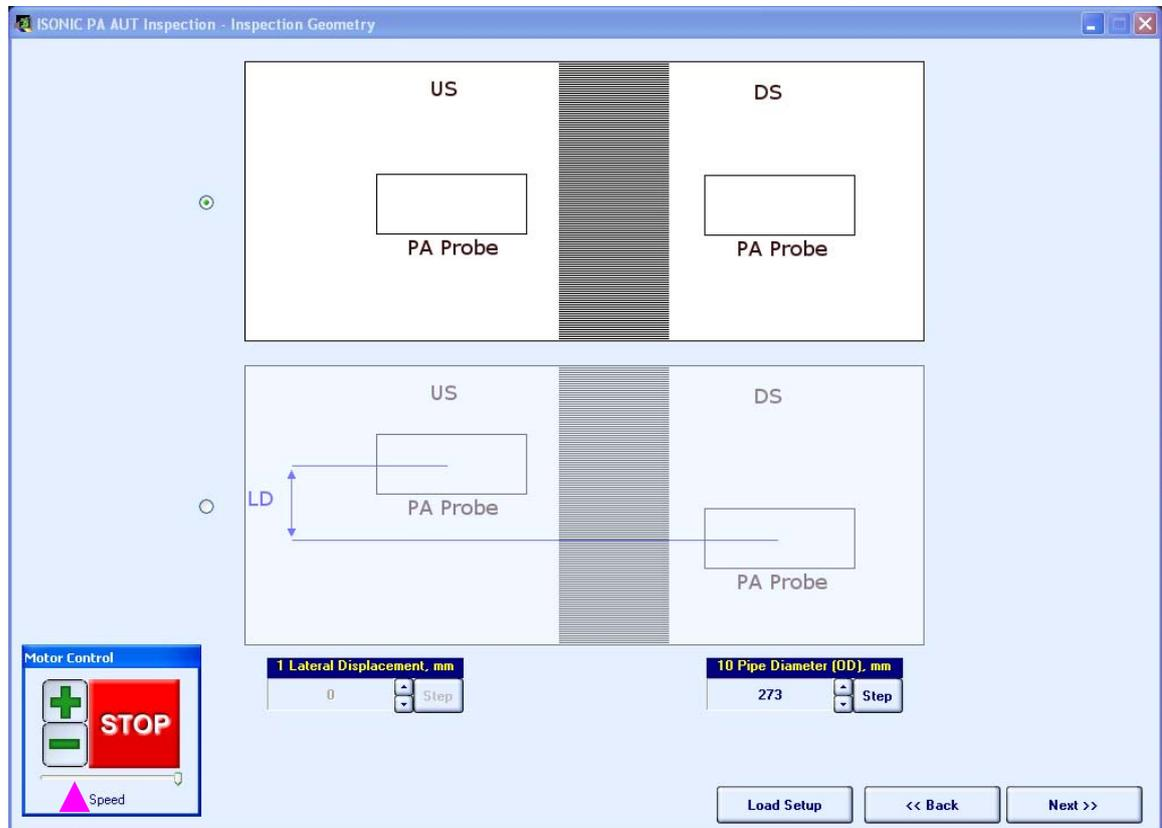
**Virtual joystick** semi-transparent control is used to place probes into cross sections containing reference reflectors precisely
