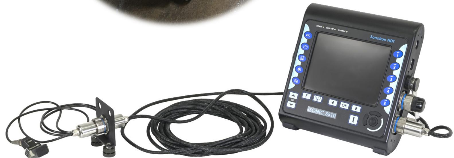
Use of detachable magnetic clamp at the probe connection side of extension cable prolongs service life of PA probes and long cable itself
