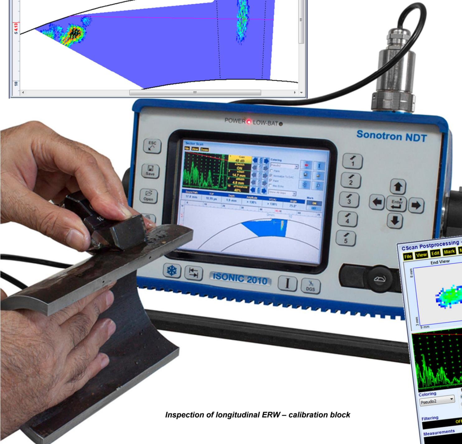
Inspection of longitudinal ERW – calibration block
