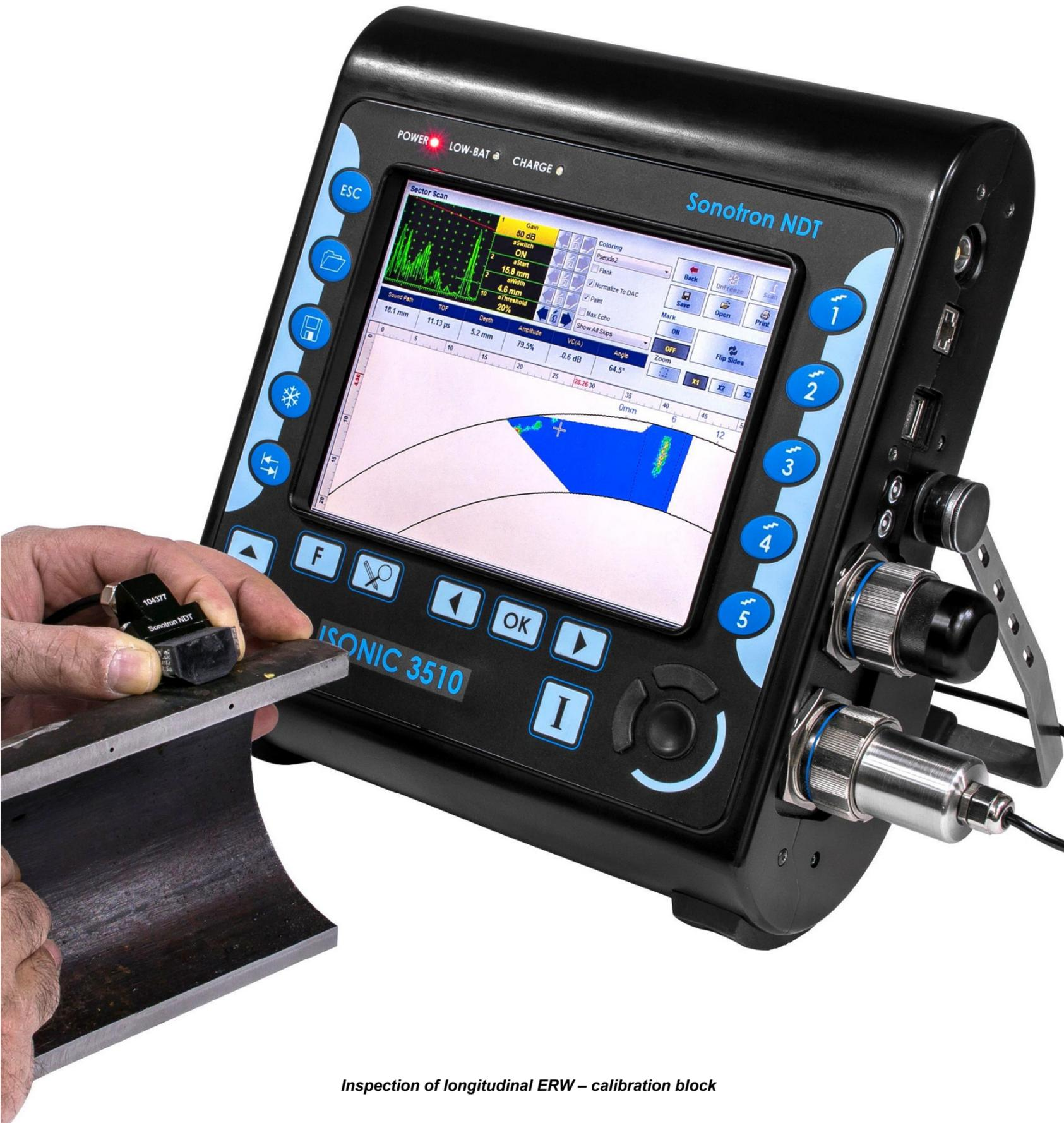
Inspection of longitudinal ERW – calibration block
