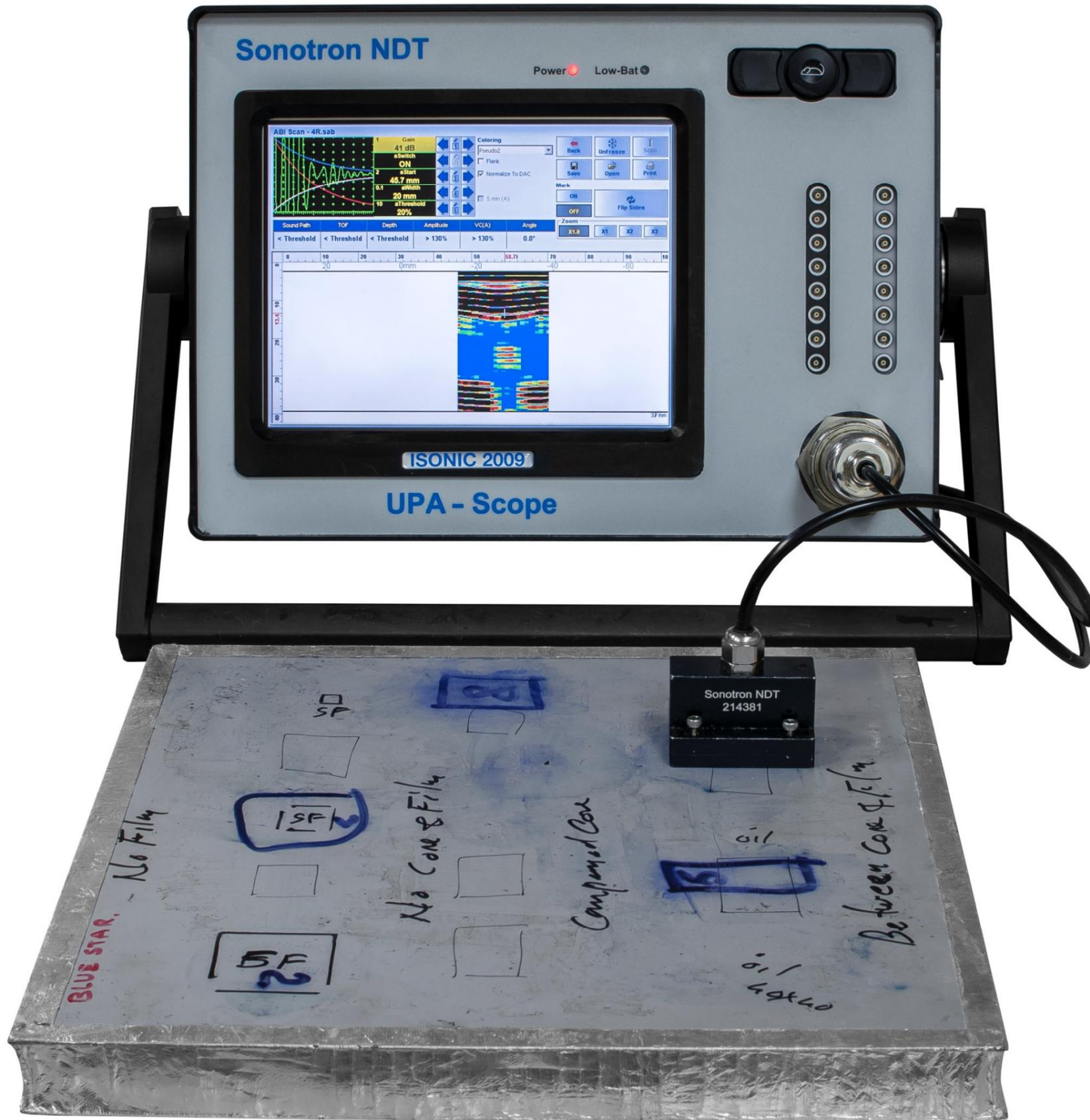
*Standard 0-deg B-Scan coverage combined with non-linear acoustic approach allowed by the powerful PA pulser receiver of ISONIC 2009 UPA Scope ensures detection of the imperfections over entire volume of the sandwich-honeycomb structure parts with use of the same high frequency highly damped PA probes, which are well suitable for the regular metals inspection*
