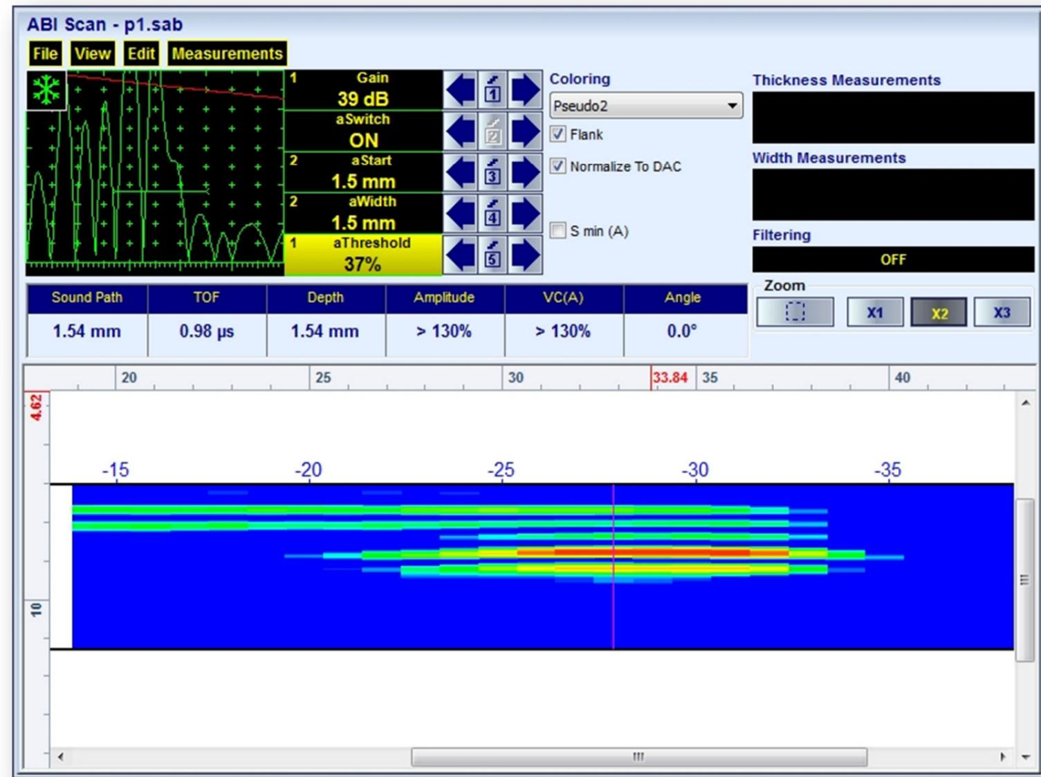
*Impact damage caused lack of bonding in the composite skin*
