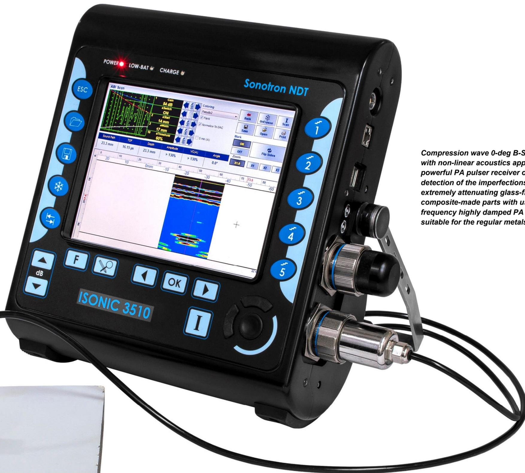
*Compression wave 0-deg B-Scan coverage combined with non-linear acoustics approach allowed by the powerful PA pulser receiver of ISONIC 3510 ensures detection of the imperfections over entire volume of the extremely attenuating glass-fiber- (GFRP) and other heavy composite-made parts with use of the same high frequency highly damped PA probes, which are well suitable for the regular metals inspection*
