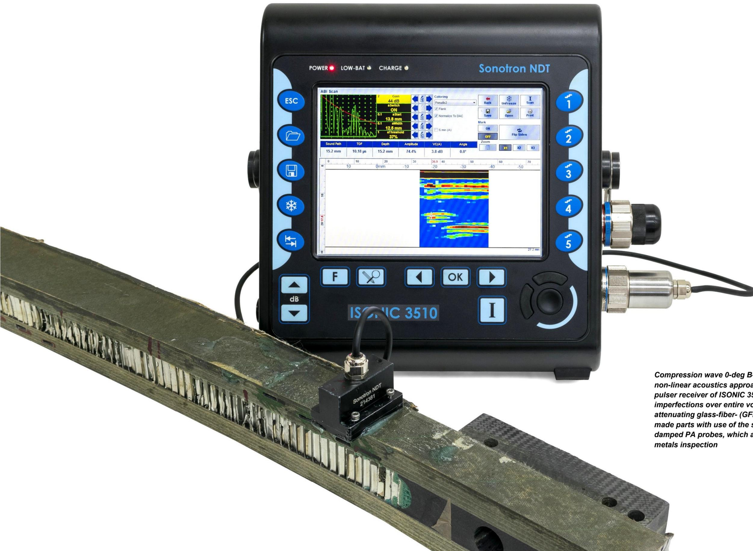
*Compression wave 0-deg B-Scan coverage combined with non-linear acoustics approach allowed by the powerful PA pulser receiver of ISONIC 3510 ensures detection of the imperfections over entire volume of the extremely attenuating glass-fiber- (GFRP) and other heavy composite-made parts with use of the same high frequency highly damped PA probes, which are well suitable for the regular metals inspection*
