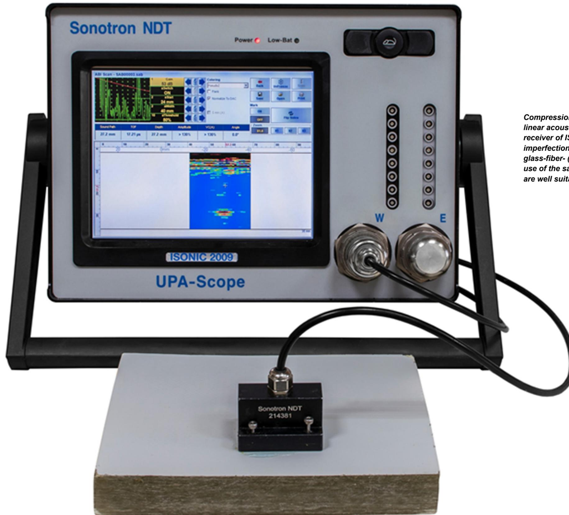
*Compression wave 0-deg B-Scan coverage combined with non-linear acoustics approach allowed by the powerful PA pulser receiver of ISONIC 2009 UPA-Scope ensures detection of the imperfections over entire volume of the extremely attenuating glass-fiber- (GFRP) and other heavy composite-made parts with use of the same high frequency highly damped PA probes, which are well suitable for the regular metals inspection*
