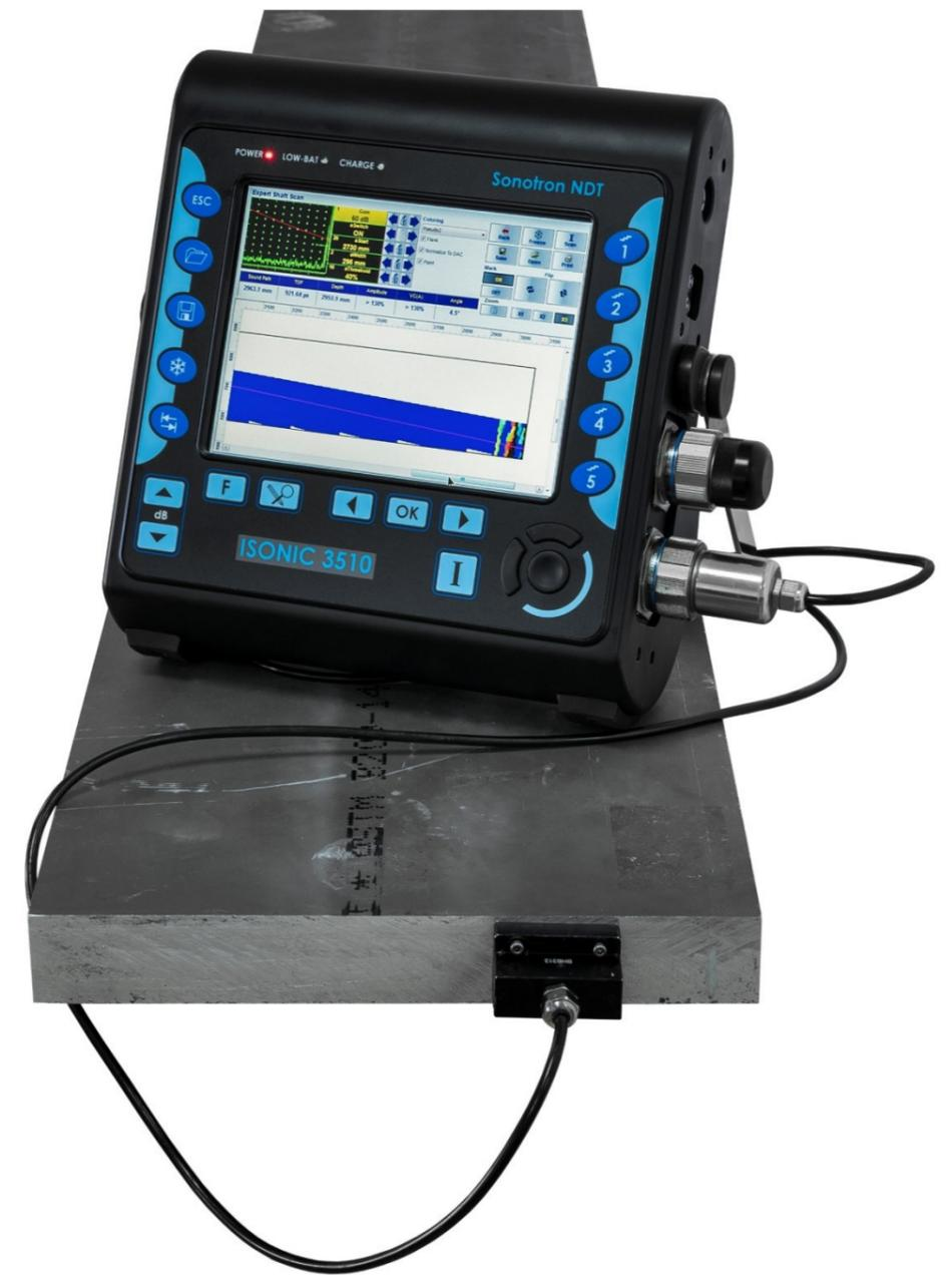
*Performance demonstration block for shaft inspection:*
