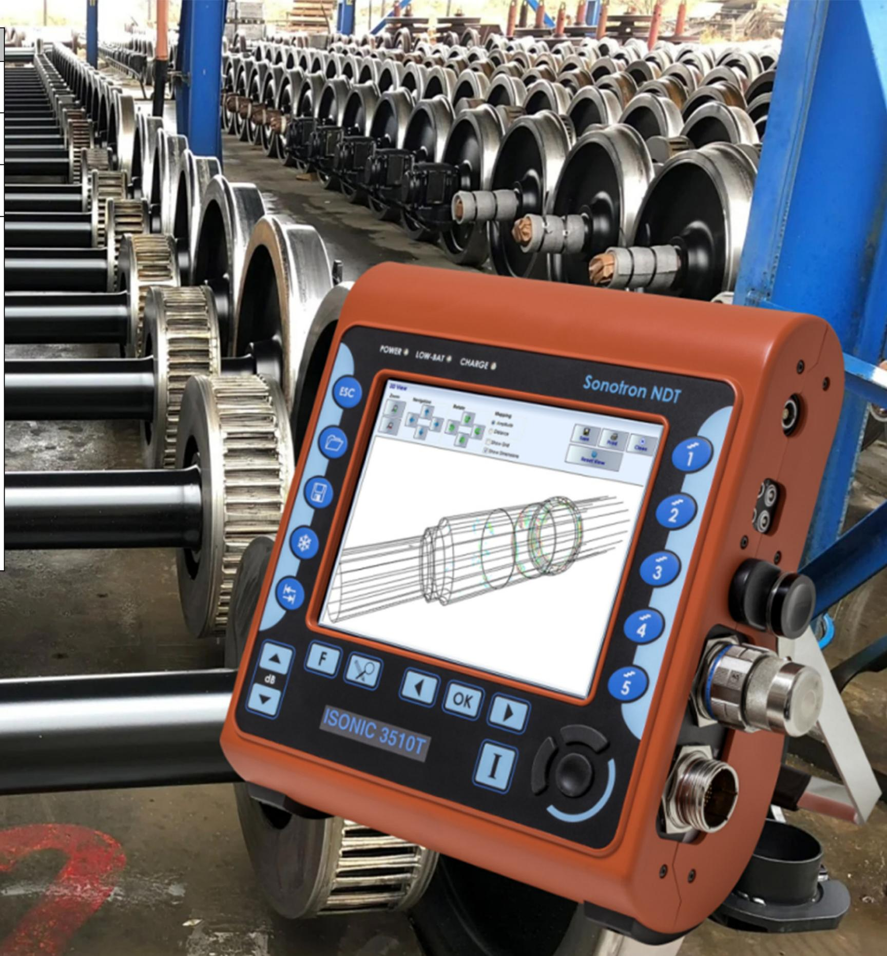
There is no disassembly of axle set required for the inspection, just the access to the end side surface of the railway axle from both sides
