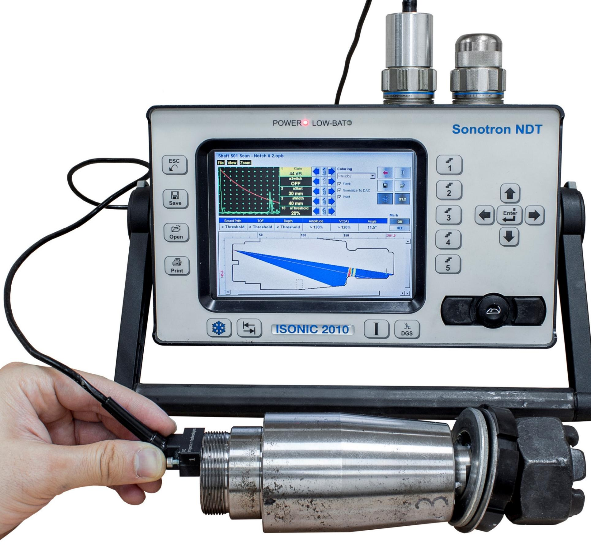
*Inspection of the complex geometry shafts*
